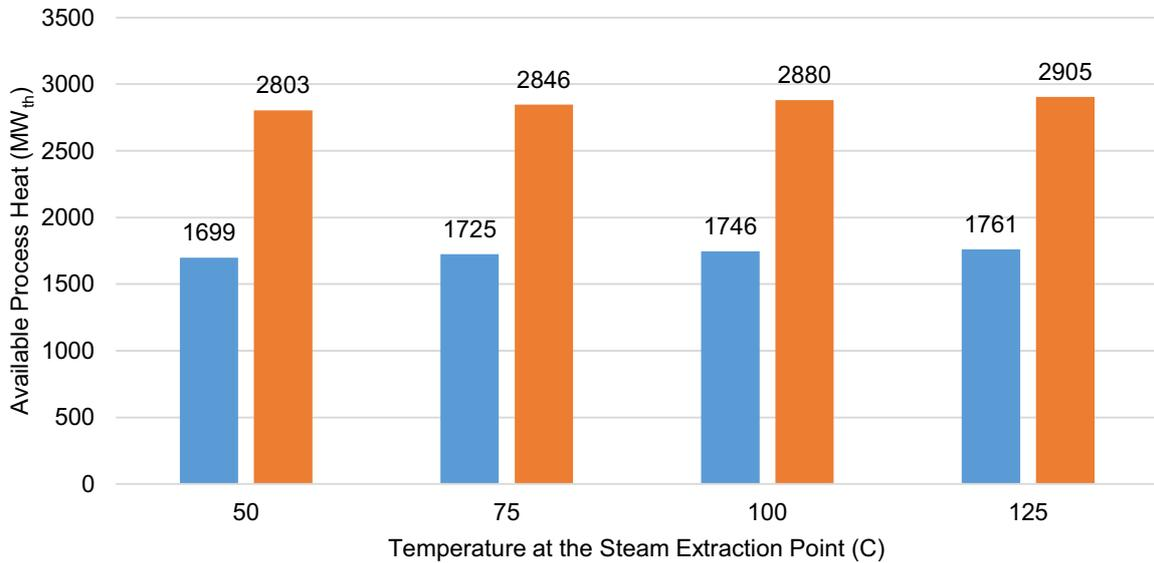
Fig. 4. Available heat for the external process vs. temperature at the steam extraction point. Blue bar: PWR 1000 MWe (2748 MW<sub>th</sub>); orange bar: PWR 1650 MWe (4534 MW<sub>th</sub>).
