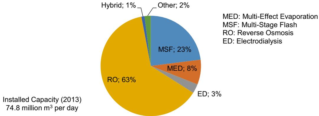
**Fig. 1.** Total worldwide installed capacity by technology.
