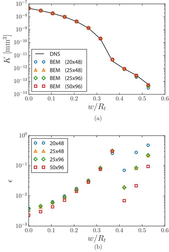
FIG. 7. Transmissivity  $K$  of the spiral-groove fracture in the  $x$  direction as a function of the dimensionless squeezing displacement  $w/R_t$ , obtained from DNS and the two-scale method (BEM) with four tessellations (a). Relative error on  $K$  obtained from DNS and the BEM for the four tiling configurations versus  $w/R_t$  (b).
