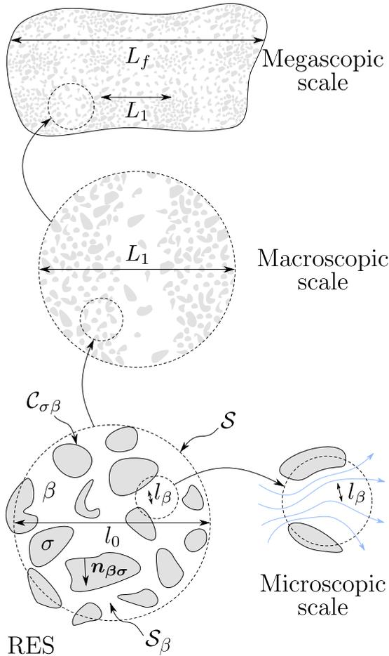
FIG. 1. Schematic view of the different scales of the fracture for the problem.  $\beta$  is the fluid phase and the contact zones are denoted by  $\sigma$ . Note that the only length-scale constraint is  $l_\beta \ll L_1$ .
