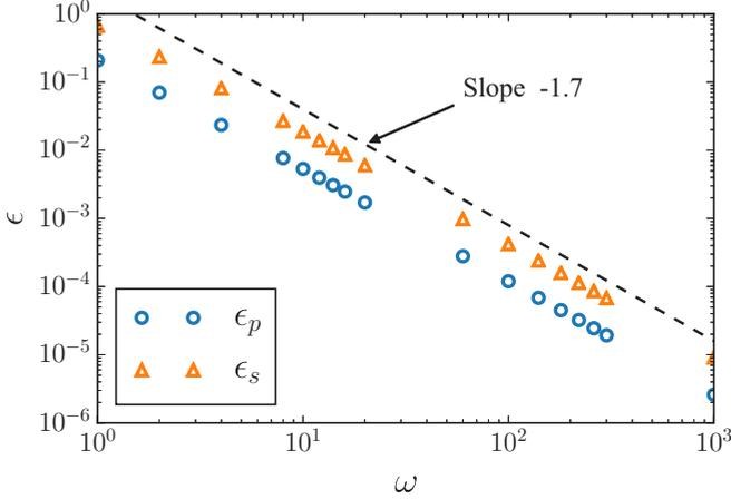
FIG. 5. Dependence of the relative error given in (37) between the analytical and computed solutions upon the mesh density  $\omega$ . The dashed line represents a power law function of  $\omega$  with an exponent  $-1.7$ .
