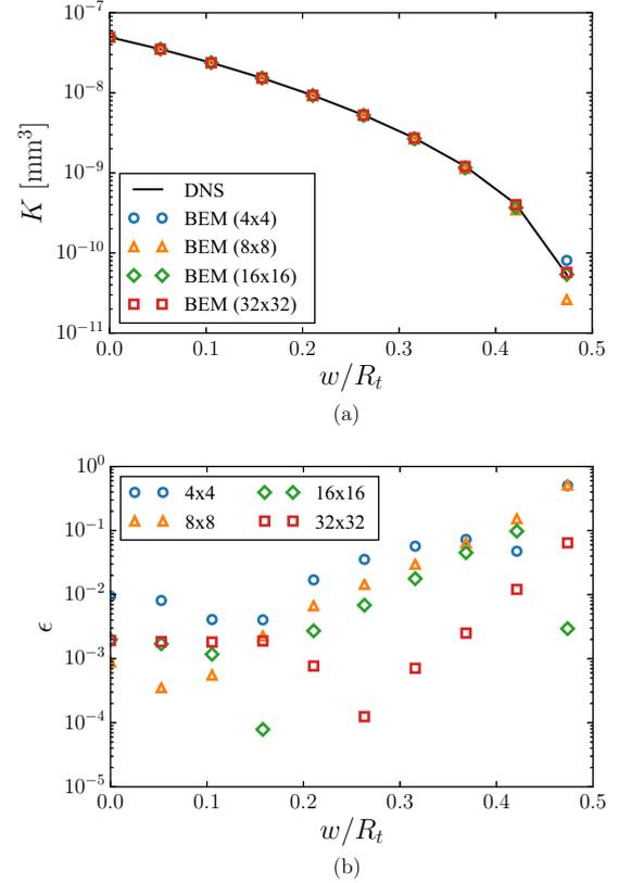
FIG. 10. Transmissivity of the fractal surface as a function of the dimensionless squeezing displacement obtained from DNS and the BEM with four tessellations (7a). Relative error on  $K$  obtained from DNS and the BEM in the four tiling configurations versus  $w/R_t$  (7b).
