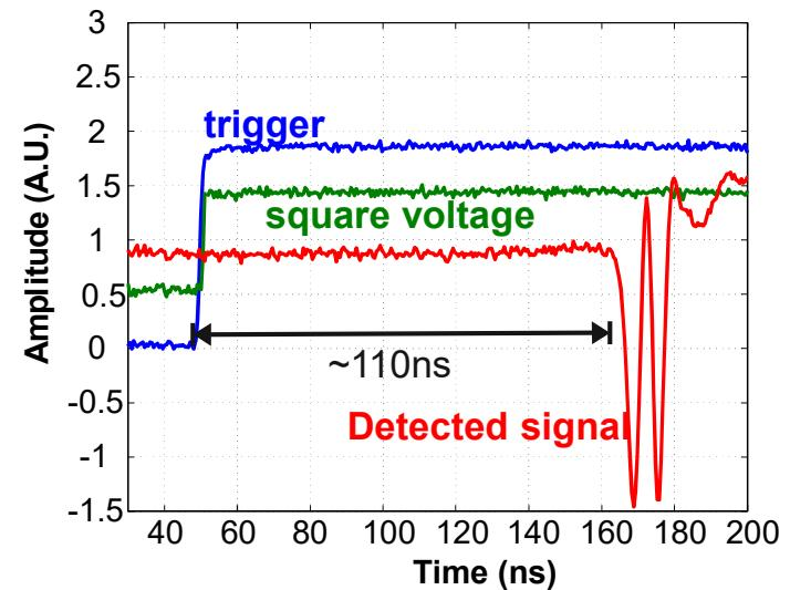
**Trigger delay  $\sim 110\text{ ns}$  (uncertainty  $\sim 2\text{ ns}$ )**
