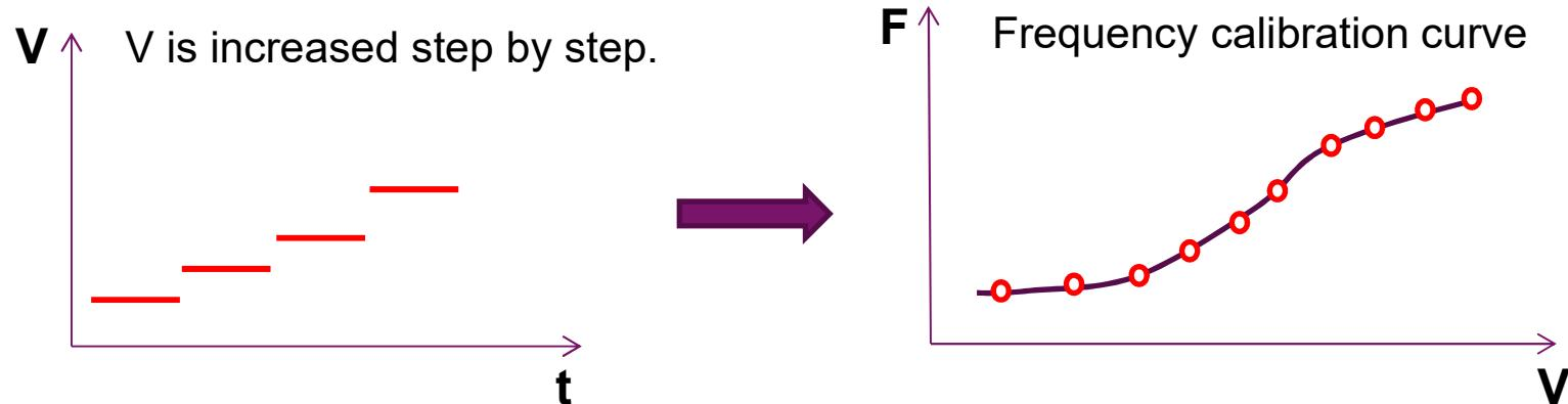
A recalculated voltage ramp is uploaded into the AWG to provide a linear frequency sweep
