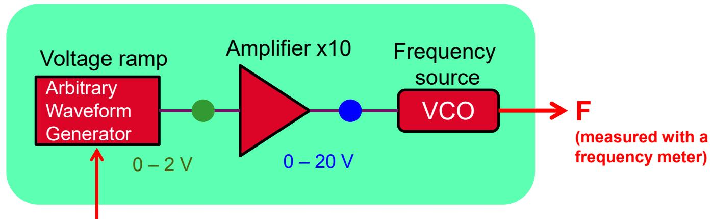
"Static" calibration procedure provides  $F(V)$
