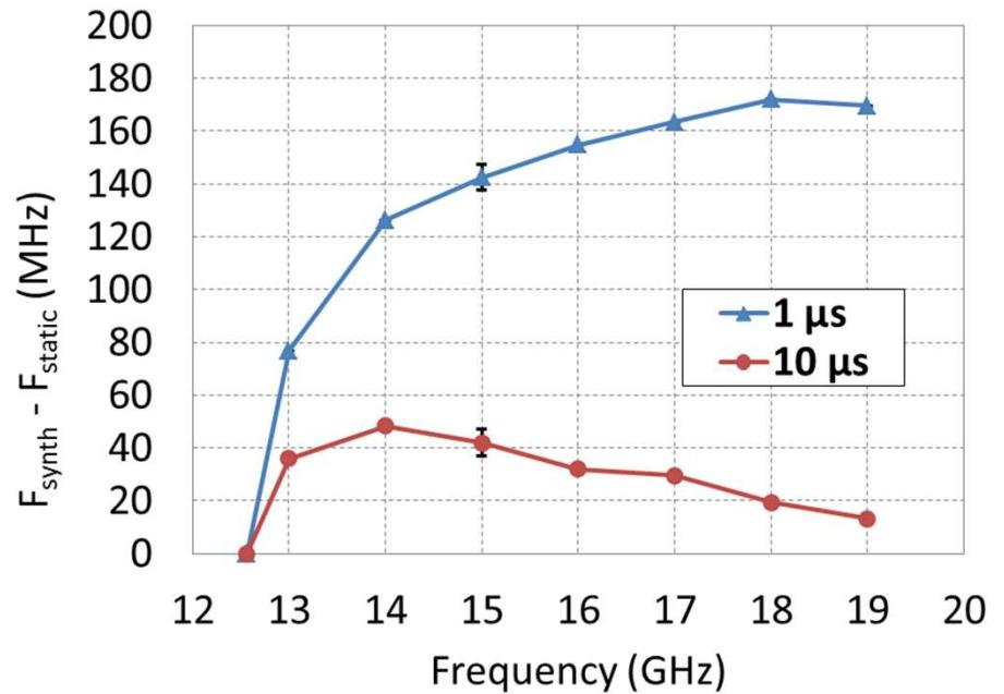
Effective probing frequencies are lower than the static calibration ones
