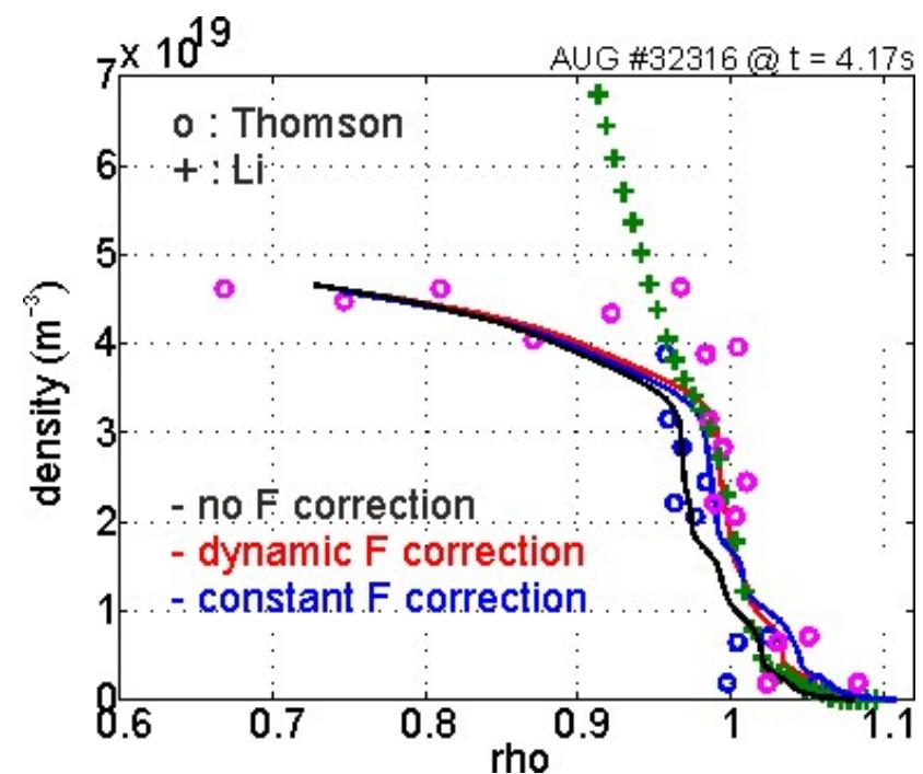
Radial shift  $\sim 1$  cm when compared to no correction.
