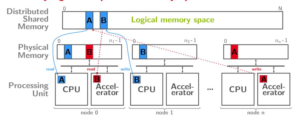
State of the art: Unifying CPU memory accesses through DSM Our objective: Allow FPGA to access to DSM
