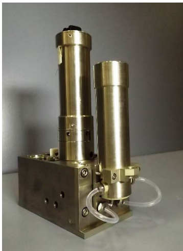
Fig. 3. Stage with recirculation pump.
