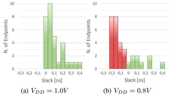
Fig. 1: Endpoint slack histogram for a 16x16-bit multiplier.
