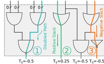
Fig. 2: Timing paths in an operator working with reduced bitwidth. Zeroed inputs are marked with a 0. Each output is associated a slack  $T_S$  computed assuming a clock period of 1 “unit”, and that all gates have a delay of 0.75 units.
