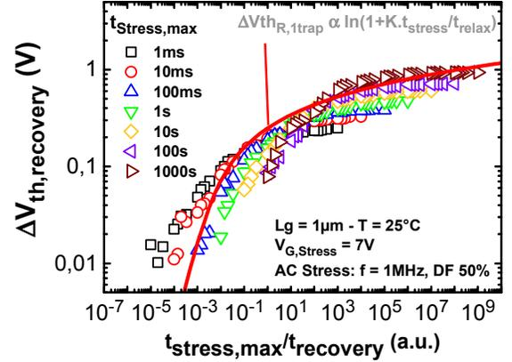
Figure 7. Recovery transients after an 1MHz AC stress plotted as a function of  $t_{Stress, MAX}/t_{recovery}$  showing no normalization, sign of multiple traps populations.  $V_{G,Stress} = 7V$  and  $L_G = 1\mu m$  here.
