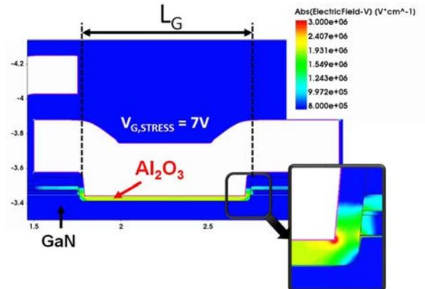
Figure 10. TCAD simulation of electric field distribution under  $V_{G,Stress} = 7V$  on 30nm  $Al_2O_3$ /GaN MOS gate stack including gate field plate and GaN-UID recess introduced in section II-A. Gate length is set at  $L_G = 1\mu m$  here. Whiteout areas are related to metallic materials.
