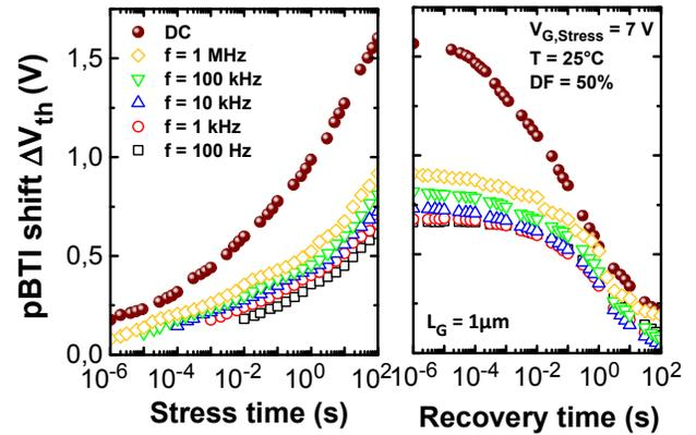
Figure 5. AC pBTI stress and recovery characteristics as a function of the signal frequency at  $\text{DF} = 50\%$ . Filled symbols represent the DC pBTI case.  $L_{\text{G}} = 1\mu\text{m}$  and  $T = 25^\circ\text{C}$  for this measurement.
