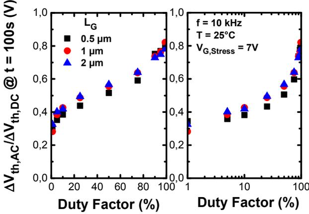
Figure 6. Variation of normalized  $\Delta V_{th,AC}/\Delta V_{th,DC}$  degradation extracted at 100s with DF. No difference with respect to gate length is observed.  $V_g = 7V$  and  $f = 10kHz$  here.
