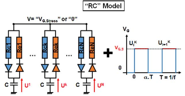
Figure 8. Schematic of the RC network used for BTI modeling [13,15]. Each traps is represented by a combination of a capacitor C and by two resistances  $R_e$  and  $R_c$  to set emission and capture time respectively. In the case of AC BTI, this circuit is studied under a  $V_g$  signal given by the chronogram (right) which gives access to the capacitor voltage  $U(t)$  after a given number of cycles.
