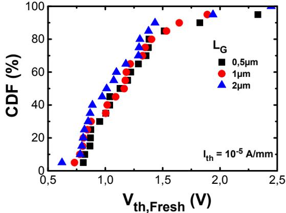
Figure 2. Cumulative distribution function of  $V_{\text{th}}$  for different  $L_{\text{G}}$  ( $0.5$ ,  $1$  and  $2\mu\text{m}$ ) confirming the E-mode operation ( $V_{\text{th}} > 0\text{V}$ ). Drain voltage is set at  $V_{\text{D}} = 0.1\text{V}$ .
