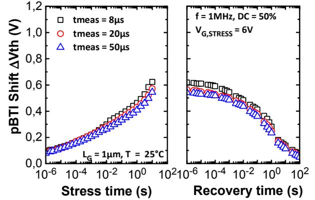
Figure 4. AC pBTI stress and recovery characteristics as a function of the  $I_{\text{D}}(V_{\text{G}})$  measurement time.  $L_{\text{G}} = 1\mu\text{m}$  and  $T = 25^\circ\text{C}$  for this measurement.
