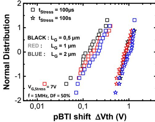
Figure 14.  $\Delta V_{th}$  distributions after two stress times (100 $\mu\text{s}$  and 100s). No visible difference is observed between 0.5 and  $1\mu\text{m}$  gate length.  $f = 1\text{MHz}$  and  $V_{G,Stress} = 7\text{V}$  here.
