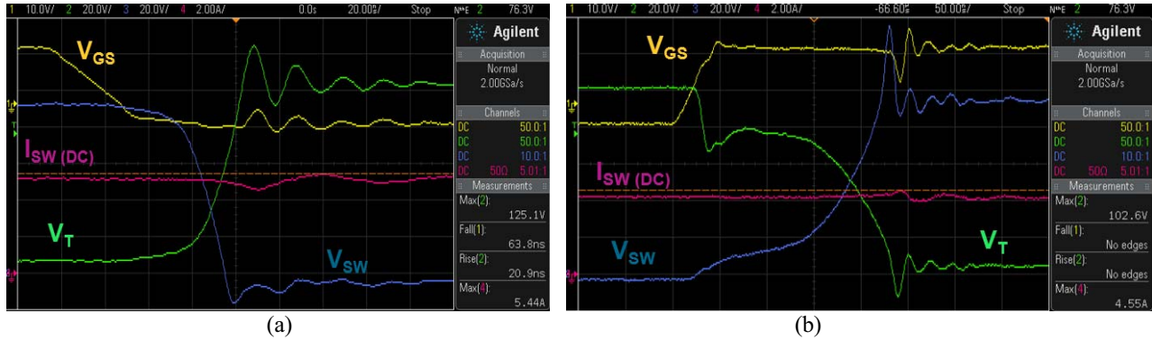
Figure 16. Dynamic characteristics of the realized 3D stack assembly at die level – V_{BUS}=100\text{ V} I_{LOAD}=5\text{ A}
