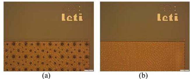
Figure 4. Top view micrograph of an AlSi serpentine patterned on top of a metallic shield with (a) or without (b) weakening structures.
