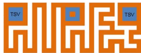
Figure 11. Example of a (lower) serpentine going from one TSV to another through a blind cavity.
