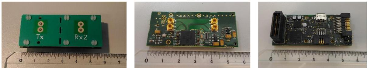
Figure 8: Antenna board (left), RF board(middle), Digital board (right)
