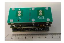
Figure 9: UWB Radar module
