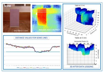
Figure 7: set-up image captures, distance measurement capabilities
