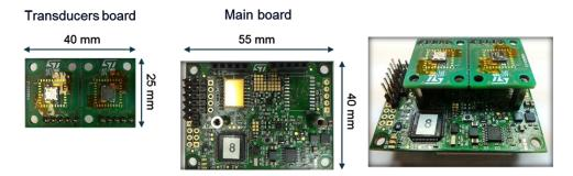
Fig. 3: Ultrasound boards for the INSPEX system
