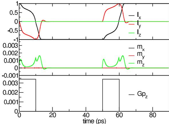
Figure 2. (Color online) Average magnetization (upper panel) and Néel order parameter components (middle panel) for uncoupled switching with parameters in reference<sup>22</sup>. The lower panel displays the STT pulses. The figures agree with the reference<sup>21</sup> because the magnetoelastic constants are set to zero.
