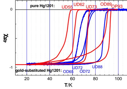
**Fig. 5.** Temperature-dependence of the normalized magnetic susceptibility of under-doped (UD), optimal (OP) and over-doped (OD) crystals of pure (red) and gold-substituted (blue)  $\text{HgBa}_2\text{CuO}_{4+\delta}$ .
