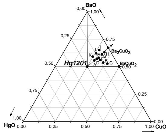
**Fig. 2.** Phase diagram for HgO-BaO-CuO in air. Our study has identified a region of low melting compositions for application of the nonstoichiometric melt method. A composition close to “K” is favorable for synthesizing Hg-1201 crystals.
