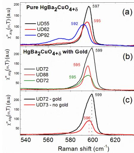
**Fig. 6.** Raman spectra of pristine and gold-substituted Hg-1201 single crystals for several doping levels.
