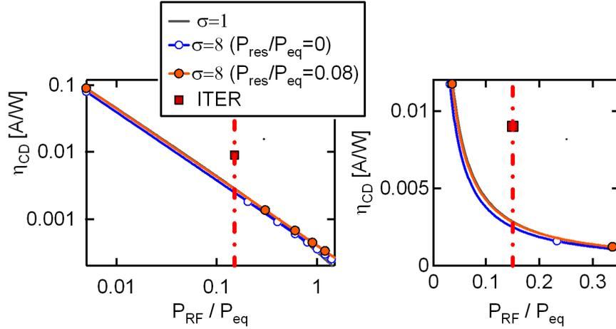
**Figure 2.** Current drive efficiency  $\eta_{CD} \equiv I_{RF}/P_{RF}$  required for (3,2) NTM stabilization as a function of the RF power ( $P_{RF}/P_{eq}$ ), with  $\sigma$  the stiffness strength, including a residual heat source  $P_{res}/P_{eq} = 0.08$  (left: log scale, right: linear scale), and we use  $W_m = 2\%$  and  $\eta_{RF}(W)$ . The ITER reference used in the numerical simulations is marked with a red square.
