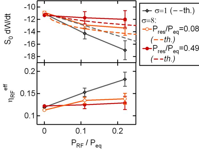
**Figure 10.** Normalized decay rate (top) and stabilization effective (bottom) averaged over the steady phase, as a function of the applied ECRH power for  $\sigma = 1$  and 8, default ( $P_{res}/P_{eq} = 0.49$ ) and ITER-like ( $P_{res}/P_{eq} = 0.08$ ) heat source.
