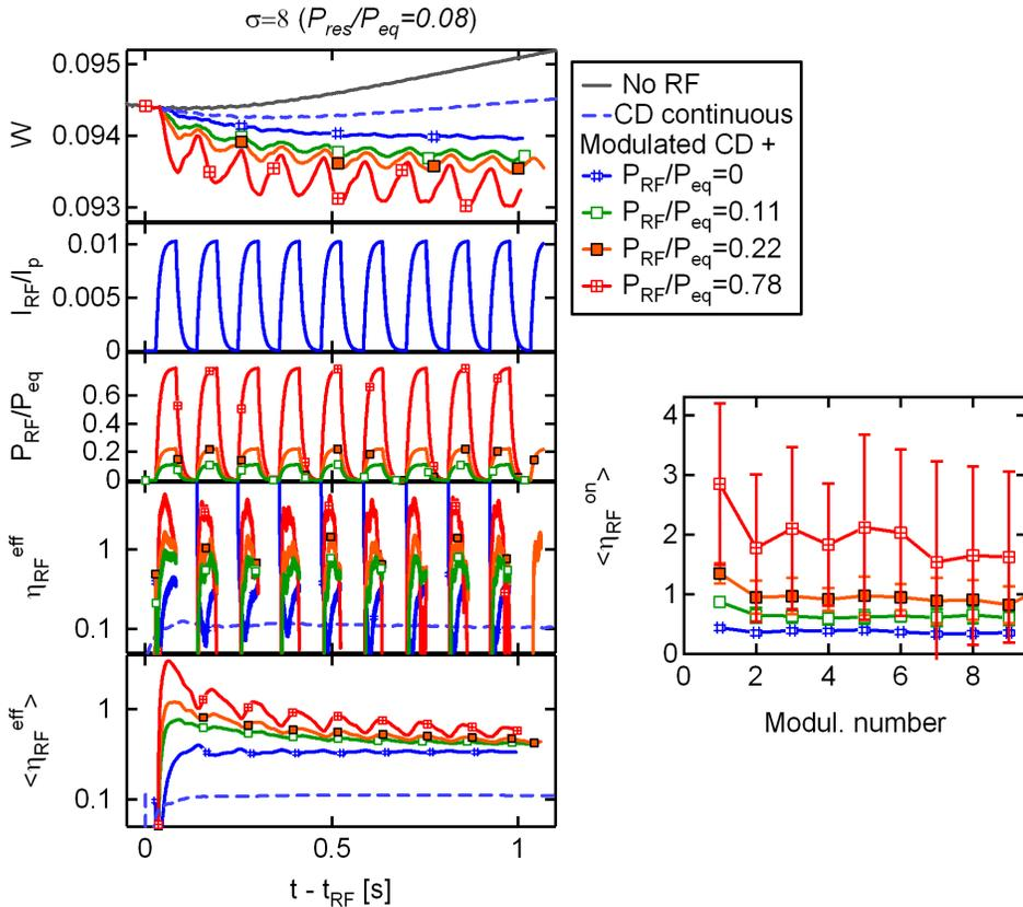
**Figure 11.** Left plot from top to bottom : island size, RF current, RF power, effective stabilization efficiency and averaged stabilization efficiency for  $\sigma = 8$  and  $P_{res}/P_{eq} = 0.08$ . Right plot: stabilization efficiency during the RF on time as a function of the modulation cycle number. The value is taken at the end of the on-time for pure RF current, and averaged over the time where the RF current is above 80% of its maximum value for the combined current and heating cases.
