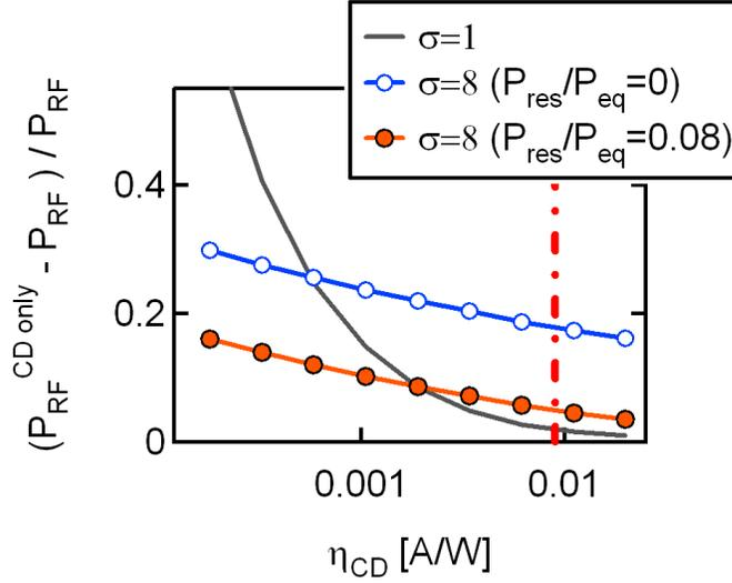
**Figure 3.** Contribution of RF heating in the stabilization of the (3,2) NTM island as a function of the current drive efficiency  $\eta_{CD} \equiv I_{RF}/P_{RF}$ . The vertical line at  $\eta_{CD} = 0.009$  is the value taken in the simulations for ITER.
