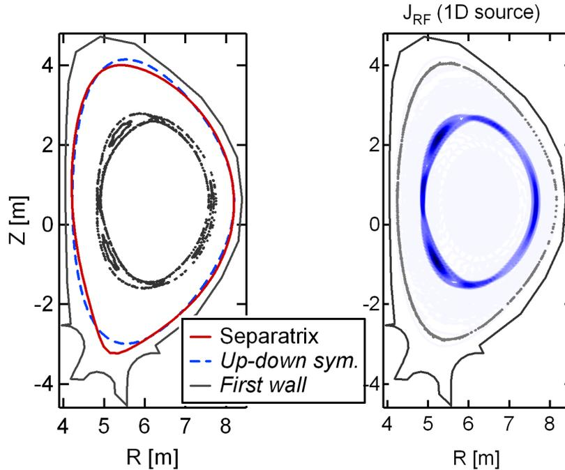
**Figure 4.** Left: plasma shape used for the simulations (up-down symmetry), with original asymmetric shape. The Poincaré plot of the (3, 2) island at saturation is also shown. Right: contour plot of the RF current density for a 1D source injected at the saturated island position.
