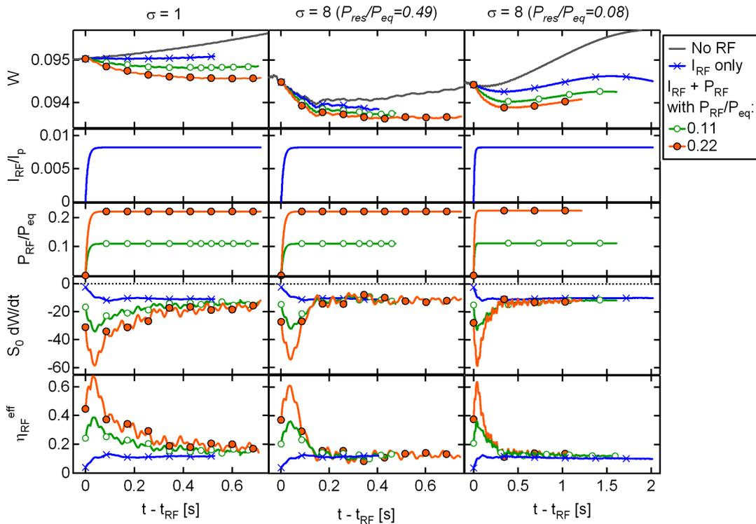
**Figure 9.** From top to bottom: island width, ratio  $I_{RF}/I_p$ , ratio  $P_{RF}/P_{eq}$ , normalized decay rate  $S_0 d\tilde{W}/dt$  and effective stabilization efficiency  $\eta_{RF}^{eff}$  for  $\sigma = 1$  (left column),  $\sigma = 8$  with a residual power inside the island of  $P_{res}/P_{eq} = 0.49$  (middle column) and  $\sigma = 8$  with a residual power inside the island of  $P_{res}/P_{eq} = 0.08$  (right column).
