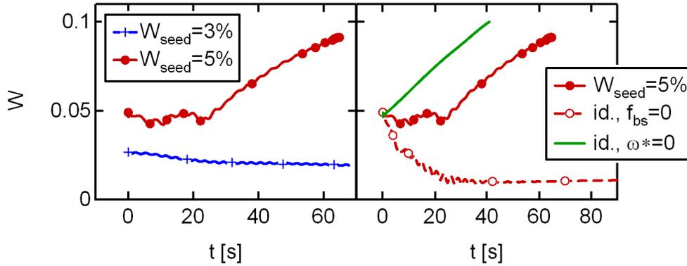
**Figure 7.** (3,2) NTM time evolution. Left: two different seed sizes, showing the metastable nature of the island. Right: simulation without bootstrap ( $J_{bs} = 0$ ) current showing that it constitutes the nonlinear drive, and without diamagnetic rotations ( $\omega^* = 0$ ) showing their stabilizing effect.
