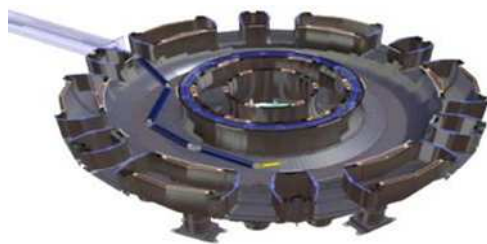
Fig. 3 - CAD view of the AIA robot performing a deployment in a Tokamak
