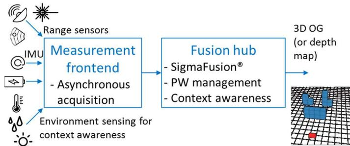
Fig. 3: INSPEX system conceptual overview (mobile detection device)
