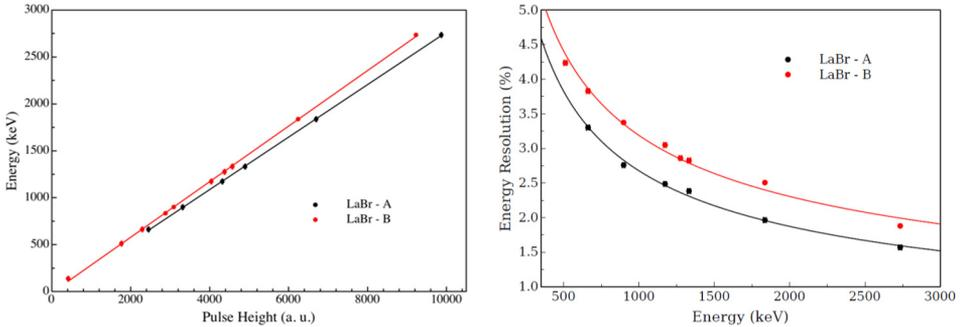
Fig. 5. (left) Energy calibrations and (right) energy resolution curves for the two 3 in  $\times$  3 in LaBr<sub>3</sub>:Ce scintillators.
