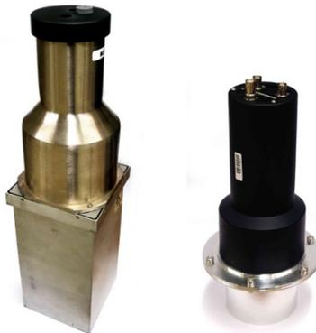
Fig. 2. View of NaI:Tl (left) and LaBr<sub>3</sub>:Ce (right) scintillators.
