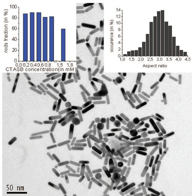
**Figure 1.** TEM picture of rods obtained with  $[\text{CTASB}] = 0.55$  mM. Right inset: aspect ratio distribution from TEM images analysis. Left inset: rod fraction (percentage in number of objects) as a function of the CTASB initial concentration from TEM image analysis.
