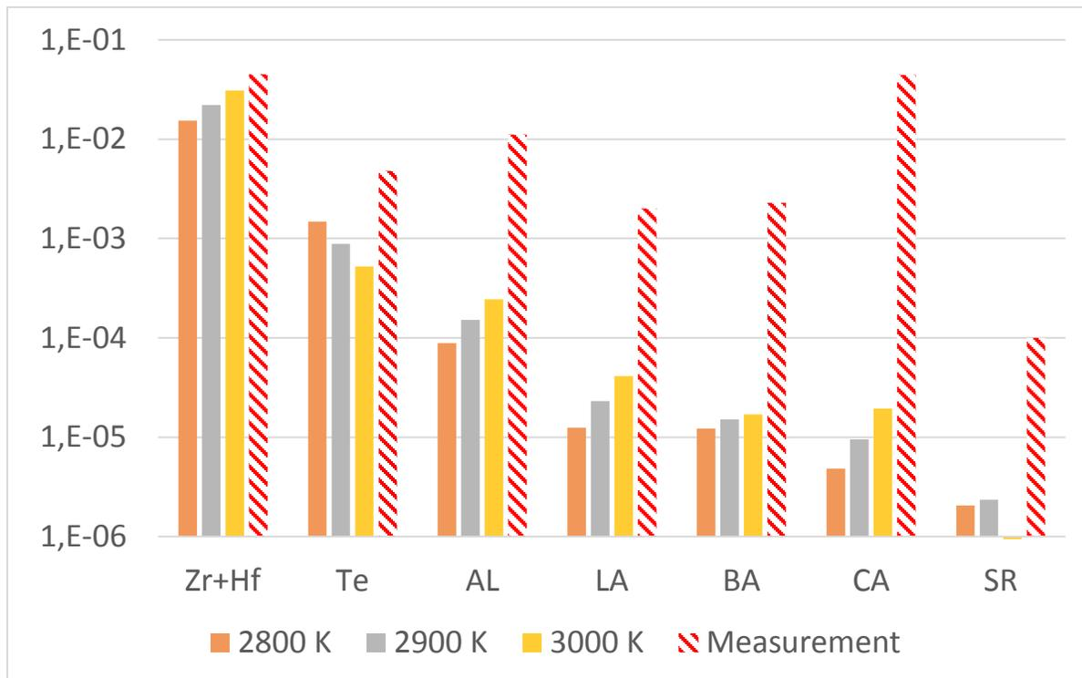
**Figure 6: Mass fractions of the minor constituents of aerosols: Calculations vs measurements**
