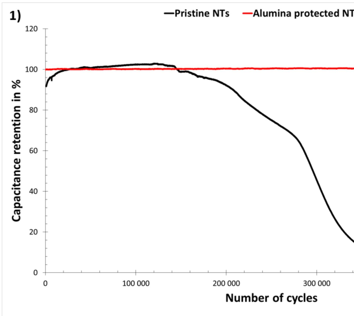
**Fig. 1** Cycling performances of Alumina protected Si NTs in  $\text{Na}_2\text{SO}_4$  at a current density of  $0.5 \text{ mA cm}^{-2}$
