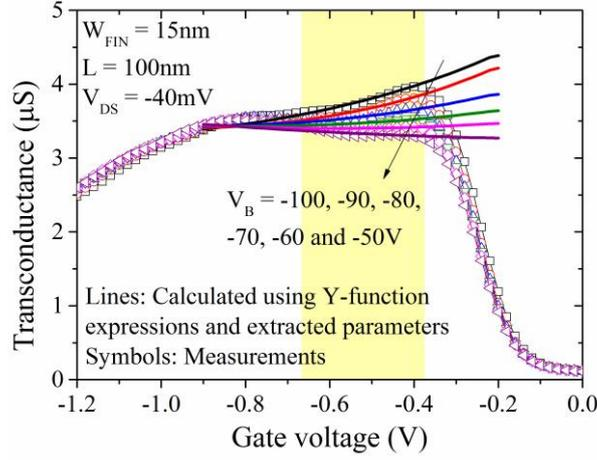
Figure 12. Step 1. Measurements and Y-function model results of  $g_m$  as a function of  $V_{GS}$  for stacked NW with  $W_{FIN} = 15\text{nm}$ ,  $L = 100\text{nm}$  and  $V_{DS} = -40\text{mV}$ . The area painted in yellow indicates the  $V_{GS}$  range chosen to apply the Y-function methodology.
