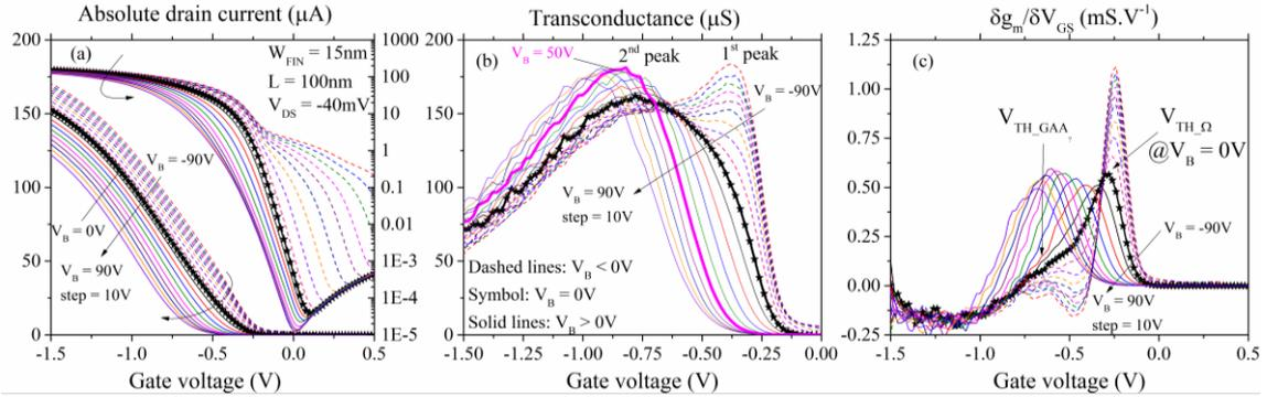
Figure 2.  $|I_{DS}|$  (a),  $g_m$  (b) and  $|\delta g_m / \delta V_{GS}|$  (c) as a function of  $V_{GS}$  for stacked NW with  $W_{FIN} = 15\text{nm}$ ,  $L = 100\text{nm}$ ,  $V_{DS} = -40\text{mV}$  and  $V_B$  from  $-90$  to  $90\text{V}$ .
