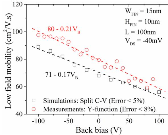
Figure 10.  $\mu_0$  as a function of  $V_{\text{B}}$  for simulated and measured non-stacked NWs with  $W_{\text{FIN}} = 15\text{nm}$ ,  $H_{\text{FIN}} = 10\text{nm}$ ,  $L = 100\text{nm}$  and  $V_{\text{DS}} = -40\text{mV}$ . Dashed lines indicate linear regression of data points, where errors obtained are smaller than 5% and 8% for simulations and measurements, respectively.
