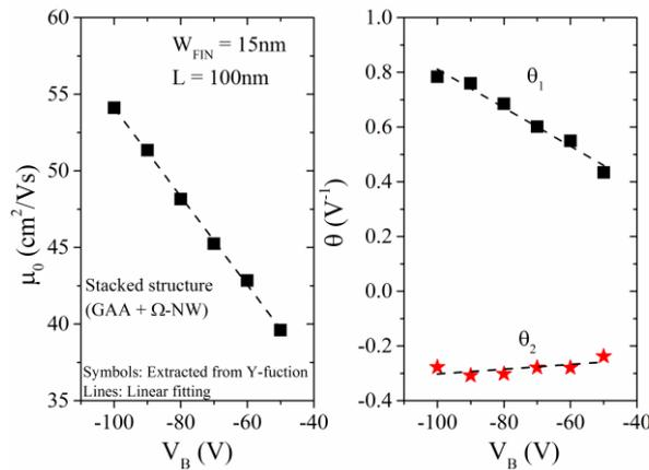
Figure 11. Step 1. Overall low field mobility (a) and mobility degradation coefficients (b) as a function of  $V_B$  for vertically stacked NWs with  $W_{FIN} = 15nm$  and  $L = 100nm$ . Results were extracted from the total  $I_{DS}$ , which corresponds to the characteristics of the whole stacked structure, i.e. sum of GAA and  $\Omega$ -NW contributions.
