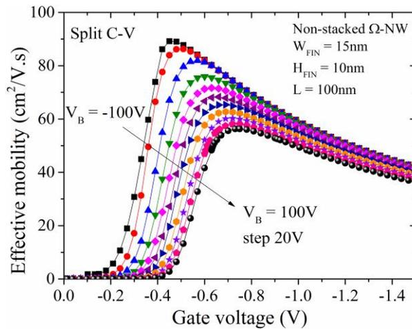
Figure 9. Simulated results for  $\mu_{\text{eff}}$  extracted by split C-V method as a function of  $V_{\text{GS}}$  for non-stacked NW with  $W_{\text{FIN}} = 15\text{nm}$ ,  $H_{\text{FIN}} = 10\text{nm}$ ,  $L = 100\text{nm}$ ,  $V_{\text{B}}$  from  $-100$  to  $100\text{V}$ .
