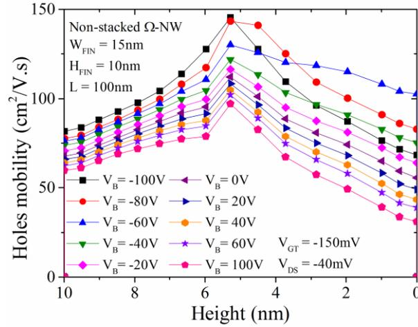
Figure 8. Simulated results for holes mobility as a function of fin height for non-stacked NW with  $W_{FIN} = 15nm$ ,  $H_{FIN} = 10nm$ ,  $L = 100nm$ ,  $V_{DS} = -40mV$ ,  $V_{GT} = -150mV$  and  $V_B$  from  $-100$  to  $100V$ .
