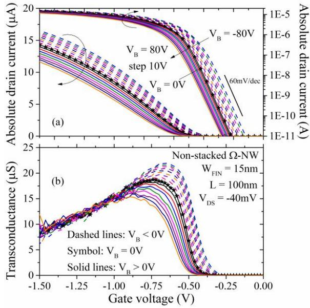
Figure 5.  $|I_{DS}|$  (a) and  $g_m$  (b) as a function of  $V_{GS}$  for non-stacked NW with  $W_{FIN} = 15\text{nm}$ ,  $L = 100\text{nm}$ ,  $V_{DS} = -40\text{mV}$  and  $V_B$  from  $-80$  to  $80\text{V}$ .
