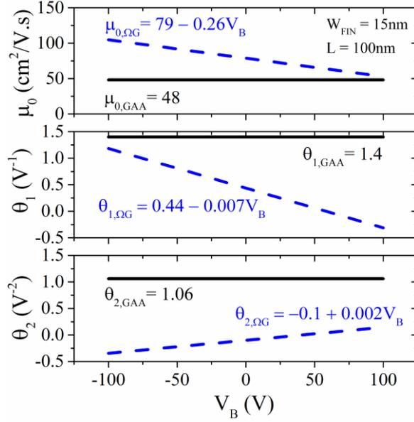
Figure 16. Parameters extracted through the proposed methodology for stacked NWs with  $W_{\text{FIN}} = 15\text{nm}$  and  $L = 100\text{nm}$ .
