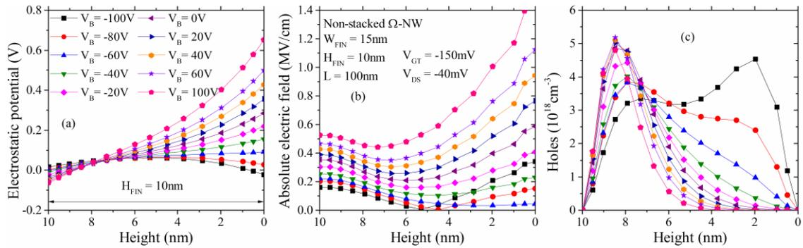
Figure 7. Simulated results for the electrostatic potential (a), electric field (b) and holes concentration (c) as a function of fin height for non-stacked NW with  $W_{FIN} = 15\text{nm}$ ,  $H_{FIN} = 10\text{nm}$ ,  $L = 100\text{nm}$ ,  $V_{DS} = -40\text{mV}$ ,  $V_{GT} = -150\text{mV}$  and  $V_B$  from  $-100$  to  $100\text{V}$ .
