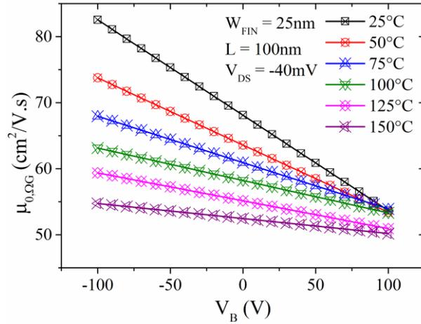
Figure 17. Extracted  $\mu_{0,\Omega G}$  as a function of  $V_B$  for bottom  $\Omega$ -NW of stacked transistor with  $W_{FIN} = 25\text{nm}$ ,  $L = 100\text{nm}$  and  $V_{DS} = -40\text{mV}$ . Temperature varies from  $25^\circ\text{C}$  to  $150^\circ\text{C}$ .
