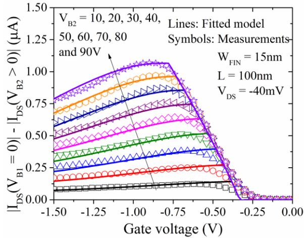
Figure 13. Step 2. Measurements and model results of  $\Delta I_{\text{DS}}$  as a function of  $V_{\text{GS}}$  for stacked NW with  $W_{\text{FIN}} = 15\text{nm}$ ,  $L = 100\text{nm}$  and  $V_{\text{DS}} = -40\text{mV}$ .
