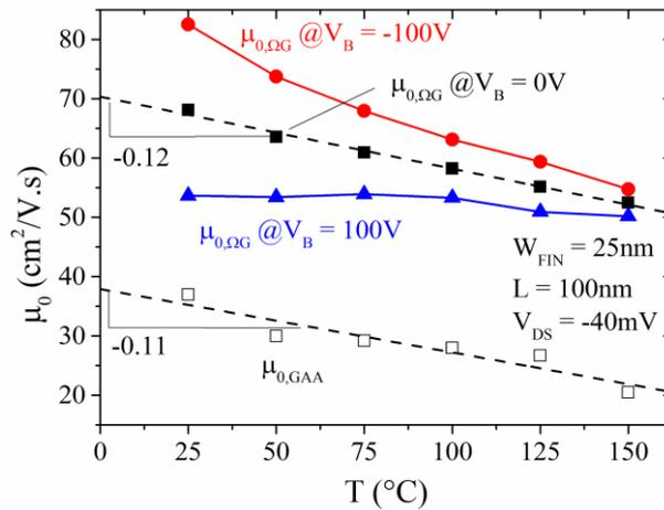
Figure 18. Extracted  $\mu_0$  as a function of  $T$  for both top GAA- and bottom  $\Omega$ -NWs of stacked transistors with  $W_{FIN} = 25\text{nm}$ ,  $L = 100\text{nm}$  and  $V_{DS} = -40\text{mV}$ . Different  $V_B$  values are shown for bottom  $\Omega$ -NW.
