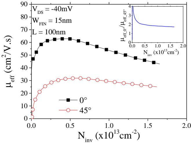
Fig.7.  $\mu_{\text{eff}}$  and  $\mu_{\text{eff}_0^\circ}/\mu_{\text{eff}_45^\circ}$  as a function of  $N_{\text{inv}}$  for [110] and [100]-NWs,  $L = 100\text{nm}$  and  $W_{\text{FIN}} = 15\text{nm}$ , at  $V_{\text{DS}} = -40\text{mV}$ .
