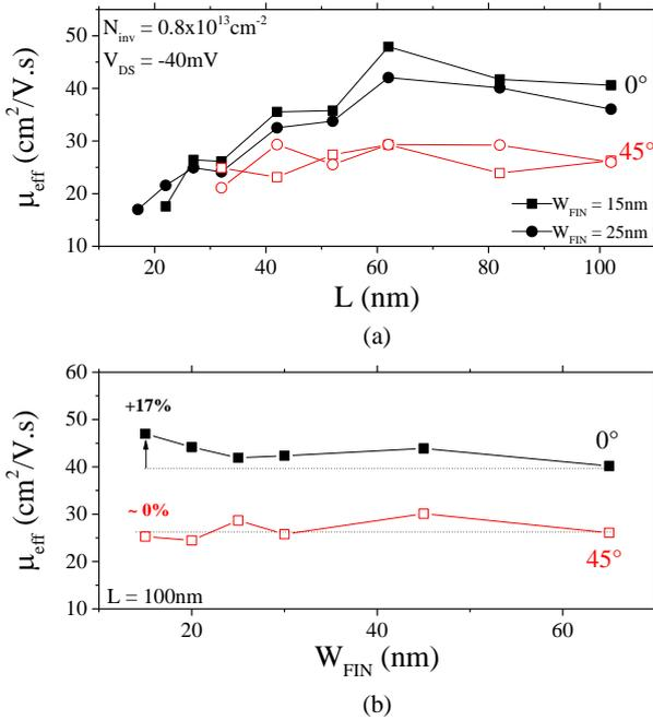
Fig.8.  $\mu_{\text{eff}}$  as a function of  $L$  (a) and  $W_{\text{FIN}}$  (b) for several [110] and [100]-NWs, at  $N_{\text{inv}} = 0.8 \times 10^{13}\text{cm}^{-2}$  and  $V_{\text{DS}} = -40\text{mV}$ .
