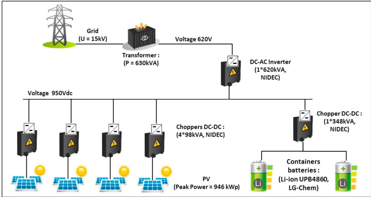
Figure 10. Electrical architecture for Li-ion (L) power plant
