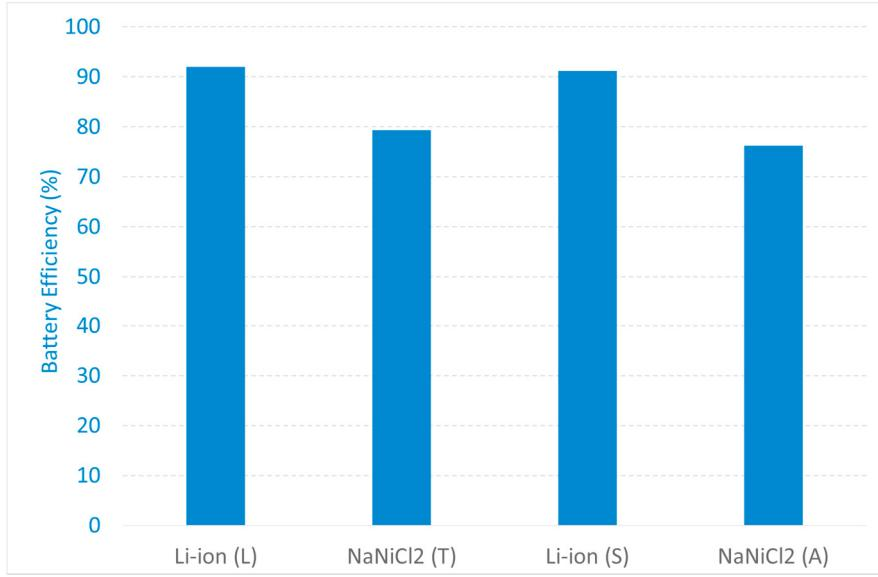
Figure 12. Yearly round-trip efficiency for 4 ESS
