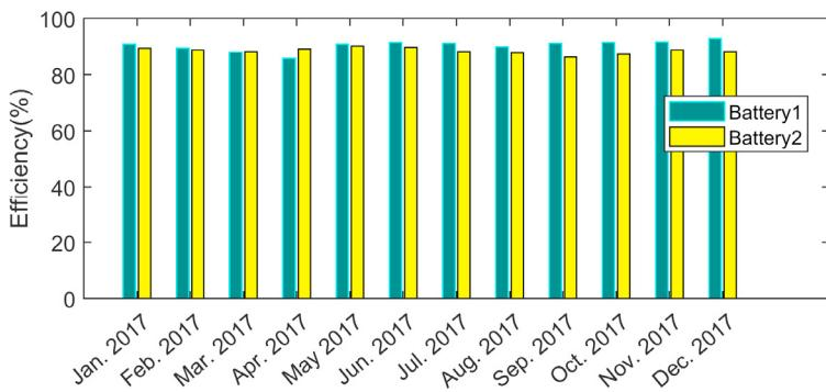
Figure 8.Annual performance indicators (round-trip efficiency of two ESS)
