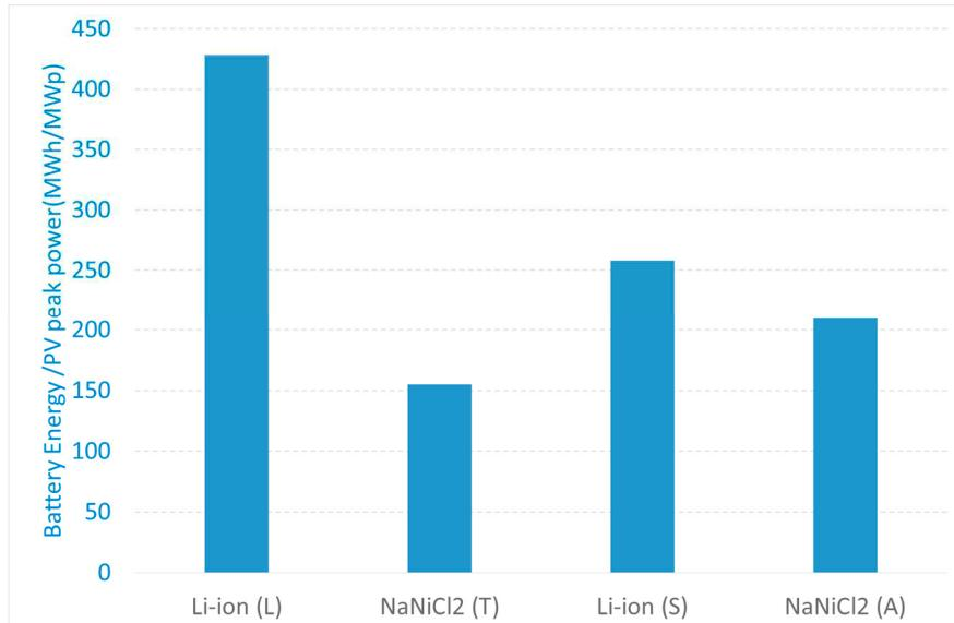
Figure 13. Yearly discharged energy for 4 ESS
