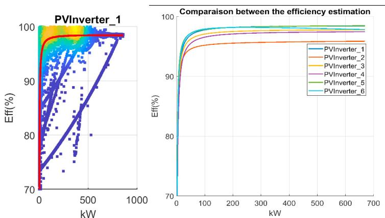
Figure 9. Power efficiency of PV inverters
