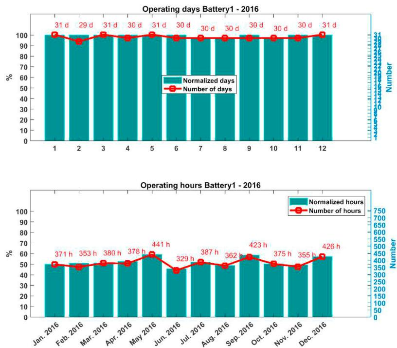
Figure 3. Battery Operation for the full year 2016
