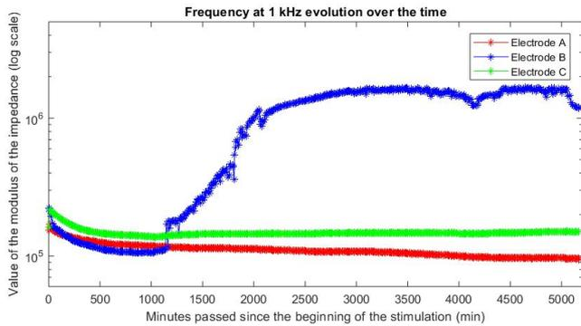
Fig. 4. Evolution of the impedance module at 1 kHz for a strip of 60 um diamond microelectrodes.
