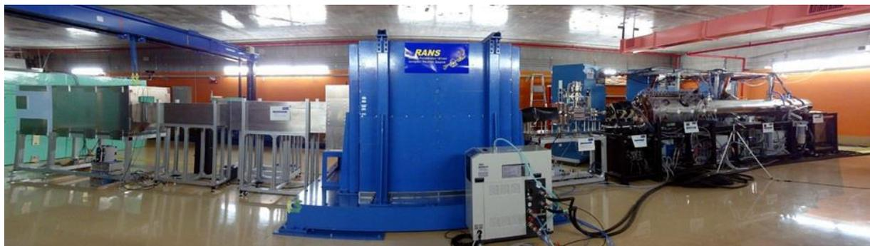
Figure 2: The RANS casemate. (left) scattering instrument (middle) TMR assembly, mostly shielding, (right) accelerator.
