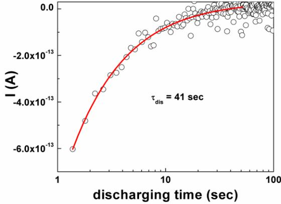
Fig. 3 Stretched exponential discharging relaxation is obtained in MIM structures
