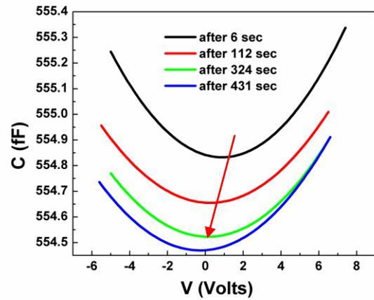
Fig. 4 C-V curves during the discharge
