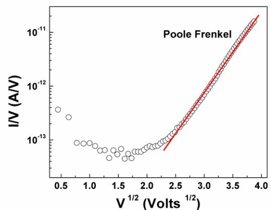
Fig. 2 Signature of Poole Frenkel conductivity for field intensities higher than 150 KV/cm
