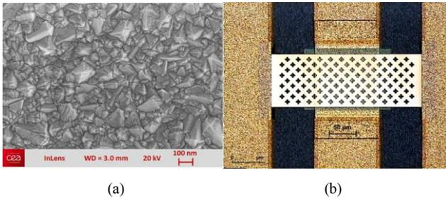
Fig.1 (a) HRSEM of the diamond film surface and (b) RF MEMS capacitive switch
