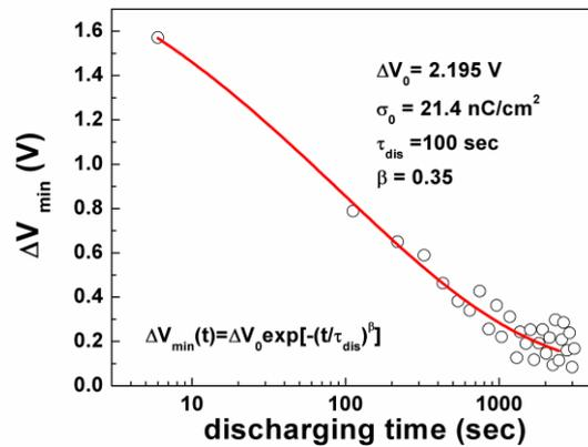
Fig. 5 Shift of  $V_{min}$  vs discharging time
