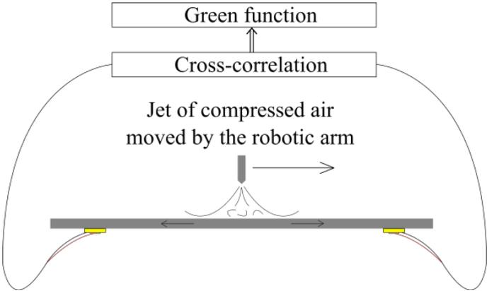
Figure 4 : Process of acquisition for passive tomography
