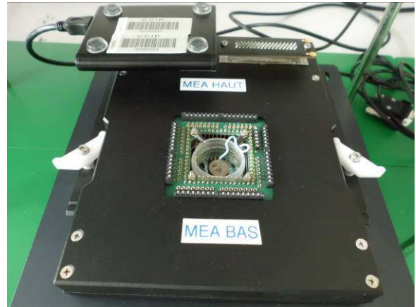
Fig. 7. A 8×8 MEA fixed on NanoZ device to measure the magnitude and phase of the electrode impedance at 1 kHz.
