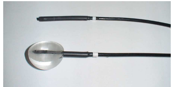
Fig. 1. OSL/FO sensor (top) and mounted with a PMMA build-up cap for surface measurements (bottom).
