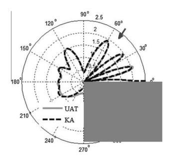
**Fig. 9.** Comparison between radiation patterns predicted by UAT and KA for a rigid wedge (gray area).  $\Phi = 270^\circ$ ,  $\theta_0 = 60^\circ$ ,  $r = 2\lambda$ ,  $\omega = 2\pi^*$  1 MHz and c = 2472 m/s. The amplitude of the total field normalized by the incident one is plotted versus the observation angle  $\theta$  in a polar diagram.
