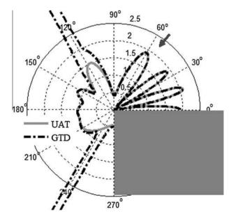
**Fig. 7.** Comparison between radiation patterns predicted by UAT and GTD for a rigid wedge (gray area).  $\Phi = 270^{\circ}$ ,  $\theta_0 = 60^{\circ}$  and  $r = 2\lambda$ ;  $\omega = 2\pi^*$  1 MHz and c = 2472 m/s. The amplitude of the total field normalized by the incident one is plotted versus the observation angle  $\theta$  in a polar diagram.
