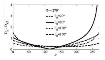
**Fig. 3.** Difference between the GTD and KA wedge diffraction coefficients for  $\Phi = 270^{\circ}$  and different incident angles  $\theta_0$ .  $\omega = 2\pi^*$  1 MHz and c = 2472 m/s.
