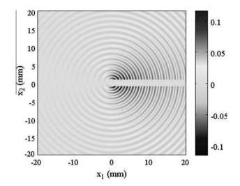
**Fig. 4.** The discrepancy between the normalized KA and exact amplitudes.  $\Phi = 360^\circ$ , incidence angle  $\theta_0 = 50^\circ$ ,  $\omega = 2\pi^* \ 1 \text{ MHz}$  and c = 2472 m/s.
