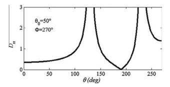
**Fig. 2.** GTD diffraction coefficient for  $\Phi = 270^{\circ}$  and  $\theta_0 = 50^{\circ}$ .  $\omega = 2\pi^*$  1 MHz and c = 2472 m/s.
