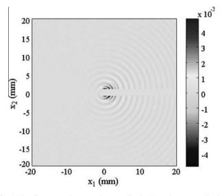
**Fig. 5.** The discrepancy between the normalized PTD and exact amplitudes.  $\Phi = 360^\circ$ ,  $\theta_0 = 50^\circ$ ,  $\omega = 2\pi^*$  1 MHz and c = 2472 m/s.
