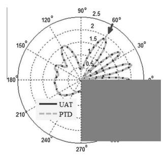
**Fig. 10.** Comparison between radiation patterns predicted by UAT and PTD for a rigid wedge (gray area).  $\Phi = 270^\circ$ ,  $\theta_0 = 60^\circ$ ,  $r = 2\lambda$ ,  $\omega = 2\pi^*$  1 MHz and c = 2472 m/s. The amplitude of the total field normalized by the incident one is plotted versus the observation angle  $\theta$  in a polar diagram.
