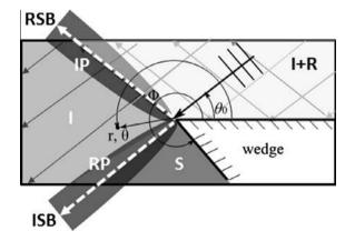
**Fig. 1.** Scatter of a plane wave incident at an angle  $\theta_0$  by a wedge of angle  $\Phi$ . Description of illuminated and shadow areas, transition zones (penumbras) and shadow boundaries (white dashed arrows).
