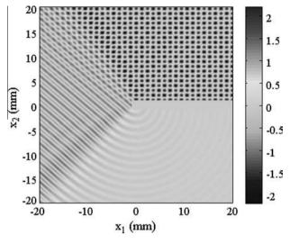
**Fig. 6.** The normalized total PTD field.  $\Phi$  = 360°,  $\theta_0$  = 50°,  $\omega = 2\pi^*$  1 MHz and c = 2472 m/s.
