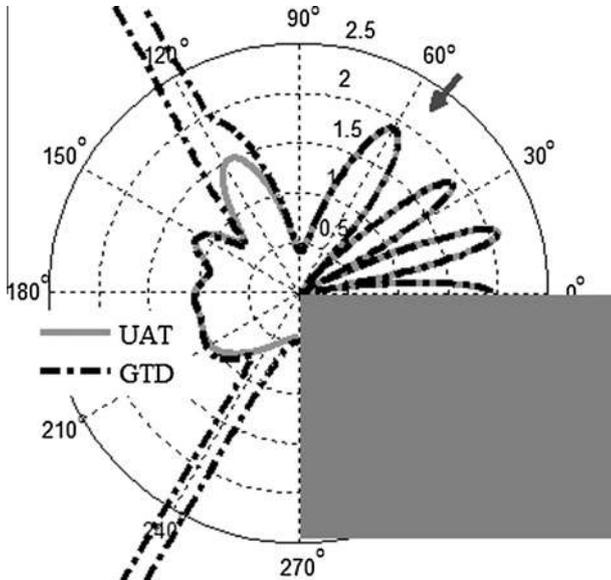
Fig. 7. Comparison between radiation patterns predicted by UAT and GTD for a rigid wedge (gray area).  $\Phi = 270^\circ$ ,  $\theta_0 = 60^\circ$  and  $r = 2\lambda$ ;  $\omega = 2\pi \cdot 1$  MHz and  $c = 2472$  m/s. The amplitude of the total field normalized by the incident one is plotted versus the observation angle  $\theta$  in a polar diagram.
