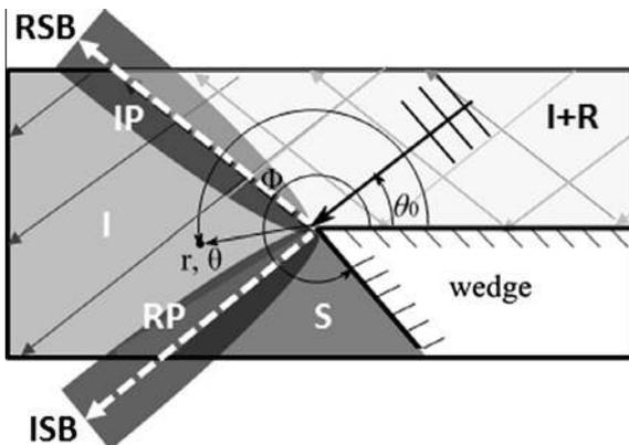
Fig. 1. Scatter of a plane wave incident at an angle  $\theta_0$  by a wedge of angle  $\Phi$ . Description of illuminated and shadow areas, transition zones (penumbras) and shadow boundaries (white dashed arrows).
