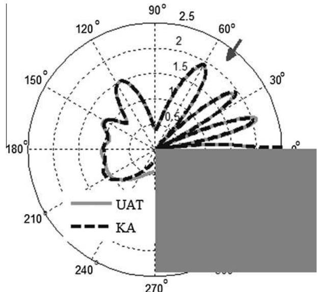
Fig. 9. Comparison between radiation patterns predicted by UAT and KA for a rigid wedge (gray area).  $\Phi = 270^\circ$ ,  $\theta_0 = 60^\circ$ ,  $r = 2\lambda$ ,  $\omega = 2\pi \cdot 1$  MHz and  $c = 2472$  m/s. The amplitude of the total field normalized by the incident one is plotted versus the observation angle  $\theta$  in a polar diagram.
