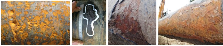
Figure 1: Example of different corrosion shapes and surfaces.
