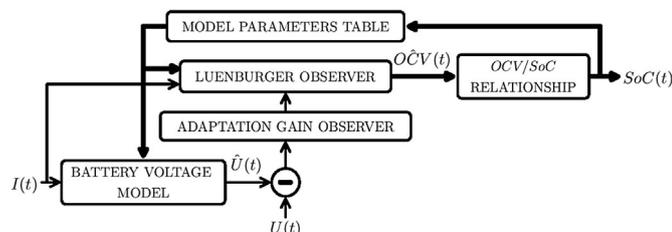
Fig. 4. SoC estimator through an adaptive Luenburger observer.
