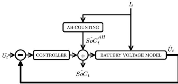
Fig. 2. Concept of SoC adjustment through a controller.
