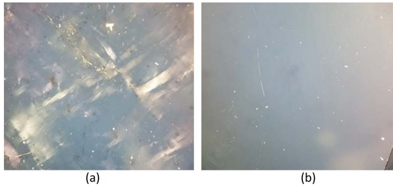
Figure 1. Crossed-polarizer optical microscopy images obtained for two ElementSix sc-CVD diamond plates: (a) electronic grade, (b) low-birefringence standard grade.
