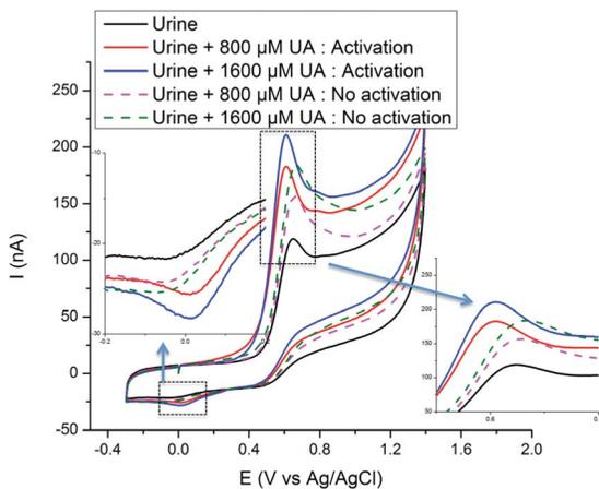
Fig. 2 Cyclic voltammograms of urine diluted 2 fold, and that of diluted urine containing added uric acid (800–1600  $\mu$ M), scanned at  $20 \text{ V s}^{-1}$ . The insets provide details of the oxidation and reduction peaks, displaying the interests of the activation process.
