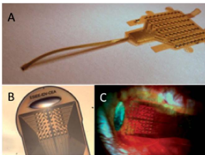
Fig. 4 (A) A view of a non-3D diamond MEA implant for retinal stimulation. The left part consists of 64 diamond electrodes as shown in (B). (C) An *in vivo* MEA array as implanted in P23H rats at the Paris Vision Institute.
