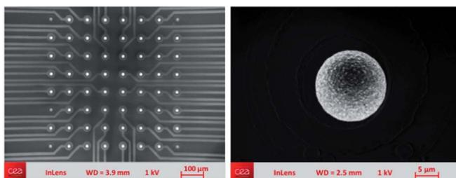
Fig. 1 Image of typical BDD diamond microelectrode arrays.
