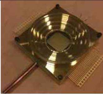
Figure 13. Specific vacuum packaging developed to integrate the bolometer FPA.
