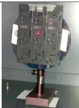
Figure 17. 3x3 metallized patterns set-up. The surface of each pattern is 4x6 cm<sup>2</sup>
