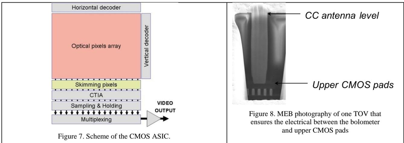
Figure 7. Scheme of the CMOS ASIC.
