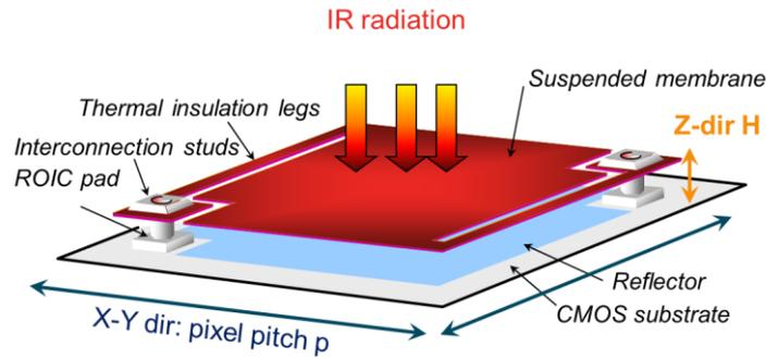
Figure 1. Scheme of a standard IR microbolometer pixel pointing out respectively the Z-direction with the suspended membrane – reflector gap height  $H$  and the X-Y directions corresponding to the pixel pitch.
