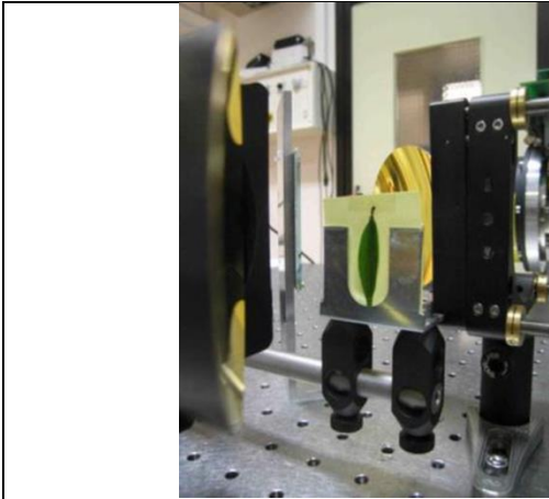
Figure 9. Laboratory set-up to image the transmission of a leaf.
