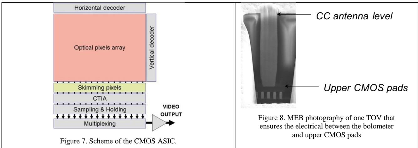
Figure 7. Scheme of the CMOS ASIC.
