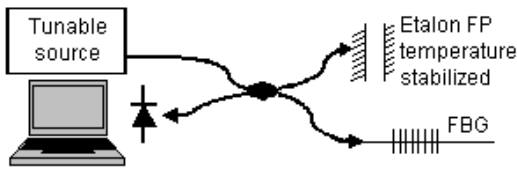
Fig. 1 Simplified diagram of the smart measurement system including the self-learning function software.
