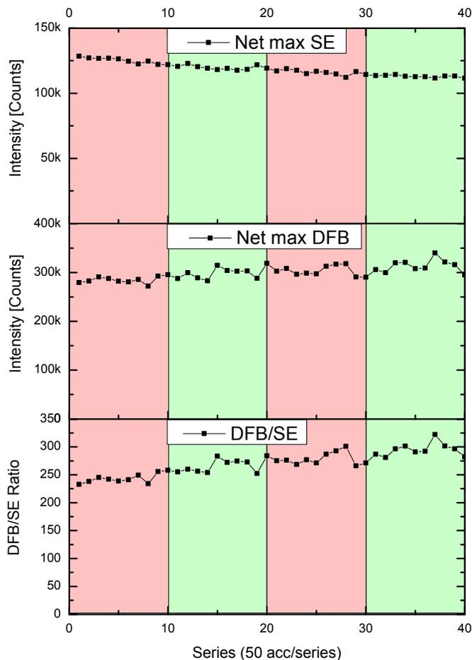
Fig. 15. DFB peak, stimulated emission continuum and ratio of the two parameters (used to normalize DFB peak value in case of input beam intensity drop) of an UGAB sample 25 MBq  $^{90}\text{Sr}/^{90}\text{Y}$  radioactive source.
