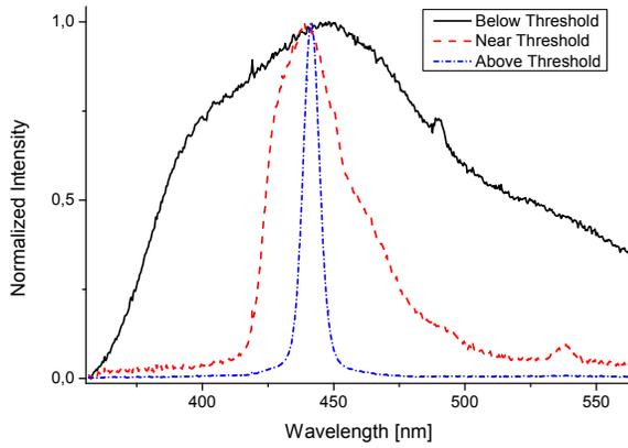
Fig. 5. Spectra showing the linewidth change between above and below stimulated emission threshold for Eljen's EJ200 plastic scintillator. Excitation beam: tripled (355 nm) pulsed picosecond  $\text{Nd}^{3+}$ :YAG laser.
