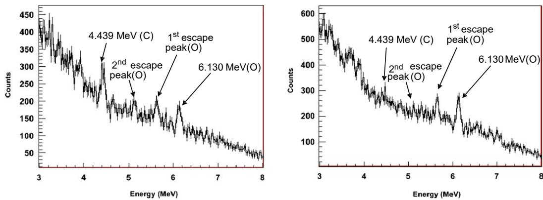
Fig. 6. Energy spectra of the 16 cm diameter and 12 mm thick iron cylinders measured for 10 min in sea water with an average neutron emission of  $2.6 \times 10^7 \text{ n s}^{-1}$  and by selecting the central alpha pixels #2, #5 and #8: the cylinder filled with  $\sim 13 \text{ kg}$  of TNT surrogate (on the left) and an identical cylinder filled with local sand (on the right).
