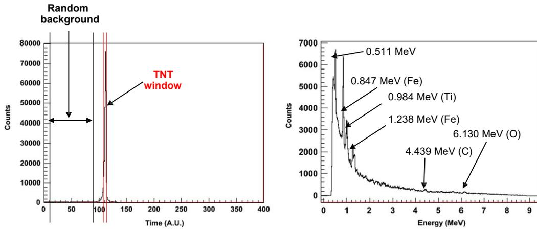
Fig. 5. TOF of the 16 cm diameter and 12 mm thick iron cylinder filled with TNT surrogate ( $C_7H_6N_3O_6$ , on the left) and energy spectra (on the right) measured in sea water for 10 min by the ROV. Average neutron emission was  $2.6 \times 10^7 \text{ n s}^{-1}$ .
