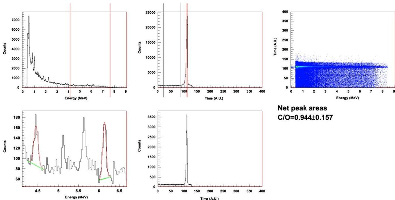
Fig. 8. Panels of the data analysis software corresponding to a 10 min measurement of the airplane bomb filled with TNT surrogate ( $\text{Si}_3\text{C}_7\text{H}_3\text{N}_3\text{O}_6$ ) in the seawater, with an average neutron emission of  $3 \times 10^7 \text{ n s}^{-1}$  and by selecting alpha pixels #3, #6 and #9.
