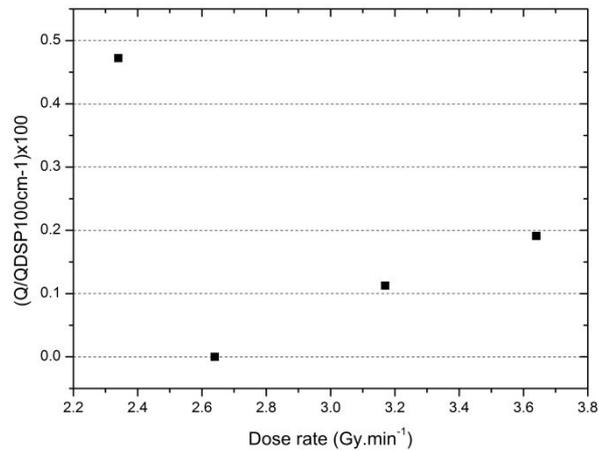
**Figure 4: Dose rate dependence of the SCDDo response in 10 x 10 cm<sup>2</sup> field, by changing the dose per pulse (SSD modification). Percentage variation of the measured charge is normalized to the value at SSD of 100 cm. Error bars are less than the height of data points (■).**
