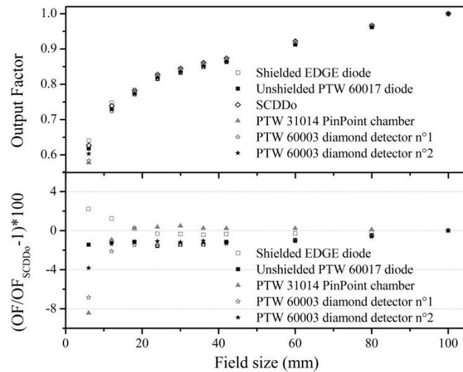
**Figure 8: (a) Output factors measured with the SCDDo, the SunNuclear EDGE diode, the PTW 60017 diode, the PTW 31014 PinPoint chamber and two different PTW diamond detectors, for 6MV photon beam, with a Varian Clinac 2100 C linac and a  $\mu$ MLC m3. Depth of measurements: 10 cm in water. SSD = 100 cm. (b) Relative difference between the commercial detectors OFs and the SCDDo OFs.**
