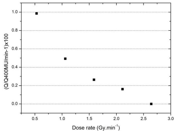
**Figure 5: Dose rate dependence of the SCDDo response in 10 x 10 cm<sup>2</sup> field, by changing the pulse repetition frequency. (a) Percentage variation of the measured charge normalized to the value at 400 MU.min<sup>-1</sup>. Error bars are less than the height of data points (■).**
