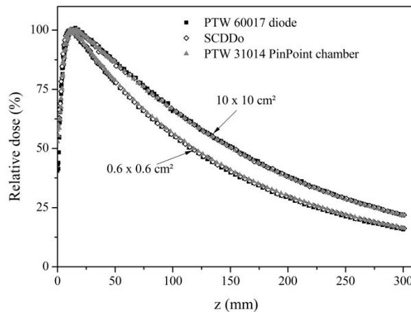
**Figure 7:** Depth dose curves measured with the SCDDo, the PTW 60017 diode and the PTW 31014 PinPoint chamber, for a 6MV photon beam, 0.6 x 0.6 cm<sup>2</sup> and 10 x 10 cm<sup>2</sup> field sizes, with a Varian Clinac 2100 C linac and a  $\mu$ MLC m3. SSD = 100 cm. Normalization at d<sub>max</sub>.
