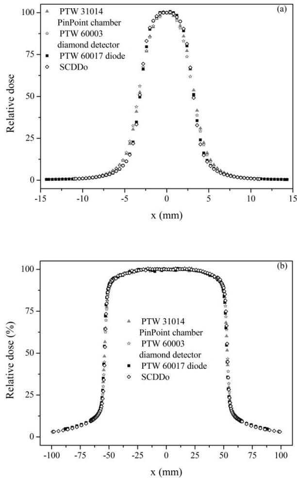
**Figure 6:** Cross-plane dose profiles measured with the SCDDo, the PTW 60017 diode, the PTW 31014 PinPoint chamber and a PTW diamond detector, for a 6MV photon beam, with a Varian Clinac 2100 C linac and a  $\mu$ MLC m3. Depth of measurements: 10 cm in water. SSD = 100 cm. Normalization on beam axis. (a)  $0.6 \times 0.6 \text{ cm}^2$  beam size. (b)  $10 \times 10 \text{ cm}^2$  beam size.
