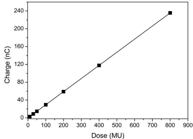
**Figure 3: Dose linearity of the SCDDo response in  $10 \times 10 \text{ cm}^2$  field at a dose rate of  $400 \text{ MU.min}^{-1}$ . Error bars are less than the height of data points (■). Linear fit is plotted with solid line.**
