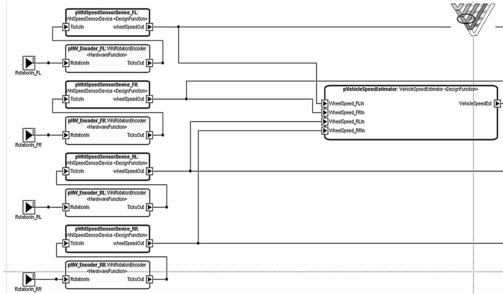
*Figure 8. Hardware architecture of the regenerative braking system*
