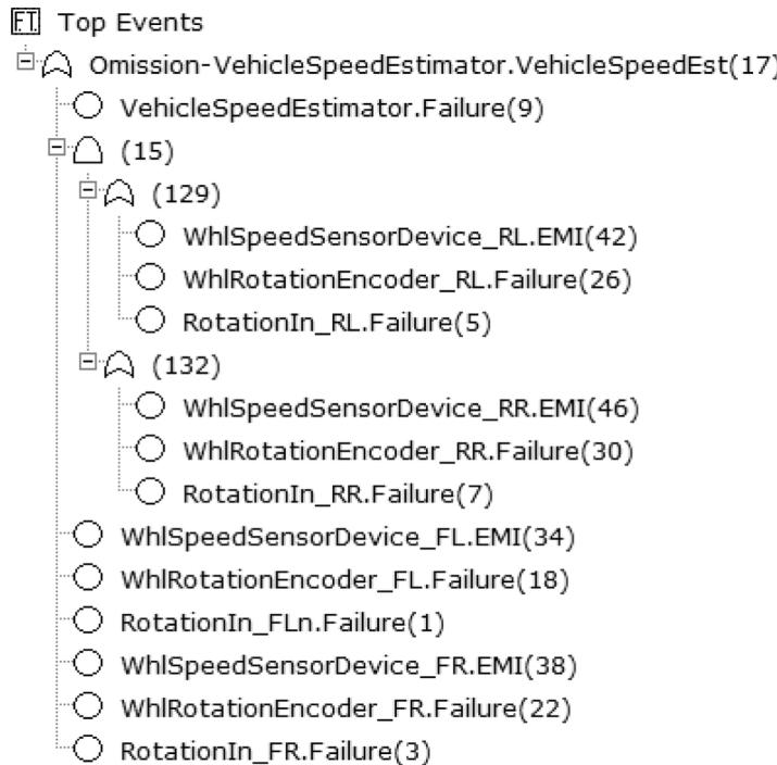
Figure 19. FMEA displayed by HiP-HOPS (excerpt)
