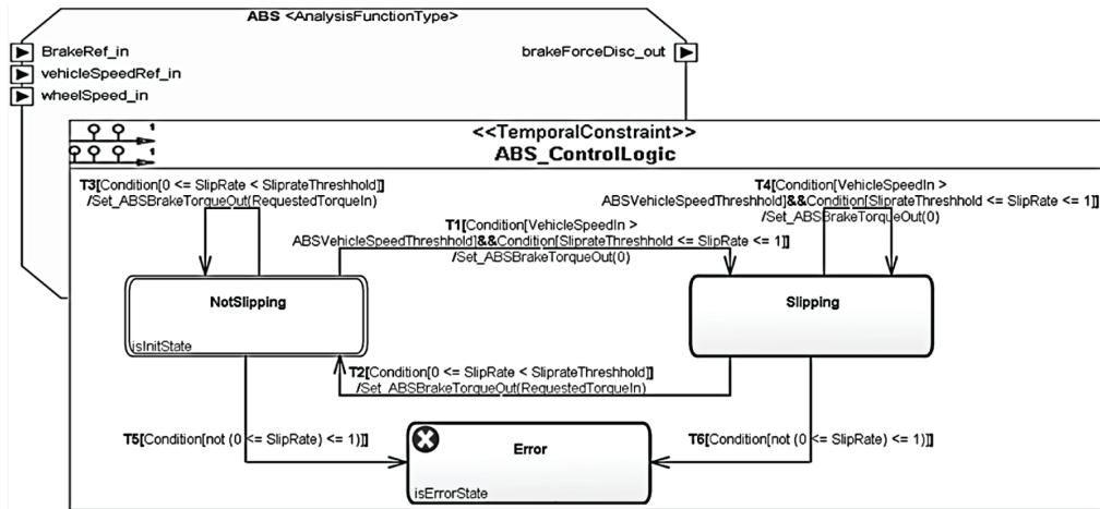
Figure 12. The computation constraint description for an ABS function
