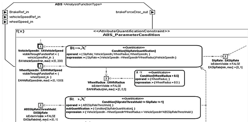
Figure 11. The temporal constraint description for an ABS function
