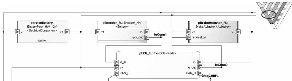
device, the ECU, the brake actuator of a wheel, and the power supply unit. The connectors among these blocks represent the electrical wires, further characterized by physical circuit properties like length, resistance and insulation. Each wire connects a pair of hardware pins (HardwarePin) of the same type, representing the electronic or electrical connection points, such as the device power pins connected to the positive pole (v+) and minus pole (v-) of the 12V DC power supply (serviceBattery).
