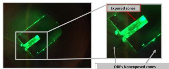
Figure 4: Fluorescence microscopy picture observed at  $\lambda_{\text{exc}}=550\ \text{nm}$  and  $\lambda_{\text{em}}=570\ \text{nm}$  of diamond cantilever functionalized with OBP immobilization after immersion in a fluorescein solution.
