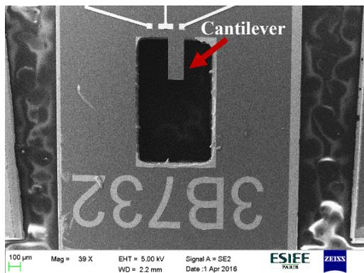
Figure 1: SEM image of a diamond micro-cantilever
