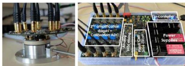
Figure 3: Gas analysis cell and electronic system
