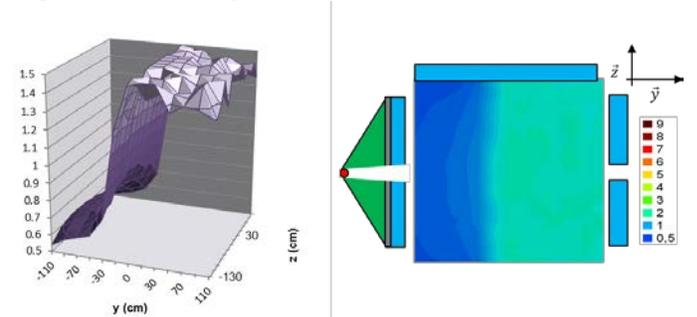
Figure 10: Ratio between three-fold coincidences of a lead block and of the bare  $0.2 \text{ g}\cdot\text{cm}^{-3}$  metallic matrix, as a function of the  $(y,z)$  coordinates of the suspicious item in the cargo container.
