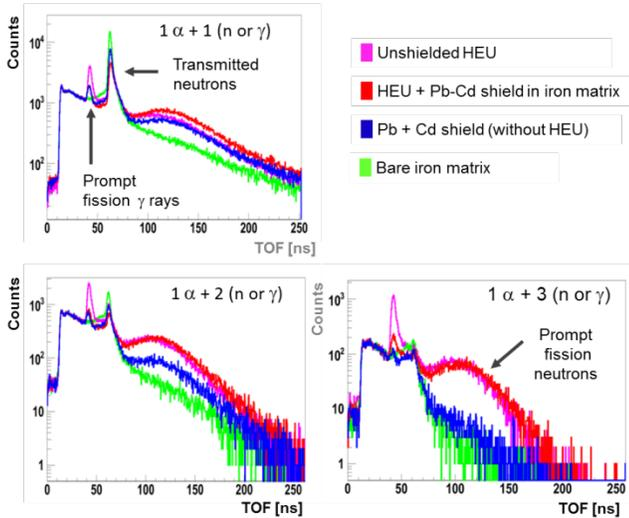
Figure 7: Simulation of a 10 min inspection of a container loaded with a  $0.2 \text{ g}\cdot\text{cm}^{-3}$  iron cargo, in which a small sample (a few kg) of HEU has been modeled in the middle of the container (unshielded: pink spectrum; shielded by lead and cadmium: red spectrum), or with the shield alone in the middle of the container (blue spectrum), or just with the iron matrix (green spectrum).
