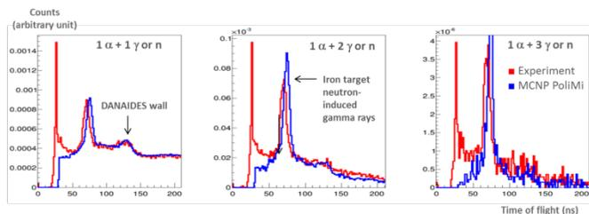
Figure 4: Time-of-flight spectra with an iron target ( $\sim 2.5 \text{ kg}$ ) inside the empty container, when an alpha particle is detected in coincidence with one, two or three gamma rays or neutrons.
