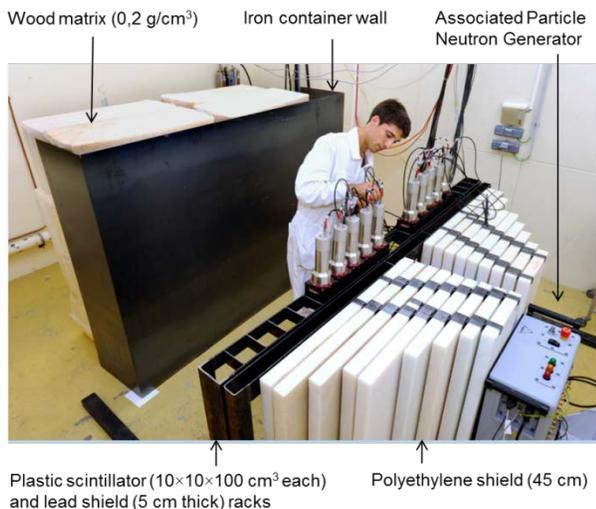
Figure 2: Experimental setup for the inspection of a container loaded with a  $0.2 \text{ g.cm}^{-3}$  wood matrix. The plastic scintillators are shielded from the generator by 45 cm polyethylene and 5 cm lead shields.
