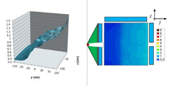
Figure 9: Ratio between three-fold coincidences of an iron block and of the bare  $0.2 \text{ g}\cdot\text{cm}^{-3}$  metallic matrix, as a function of the  $(y,z)$  coordinates of the suspicious item in the cargo container.
