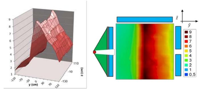
Figure 8: Ratio between three-fold coincidences in the fission neutron time window, for the shielded HEU item and for the bare  $0.2 \text{ g}\cdot\text{cm}^{-3}$  metallic matrix, respectively, as a function of  $(y,z)$  coordinates of the suspicious item in the cargo container. The depth  $y = -110 \text{ cm}$  corresponds to the first wall of the container (close to the neutron generator, red point on the 2D projection), and  $y = +110 \text{ cm}$  corresponds to the second wall.
