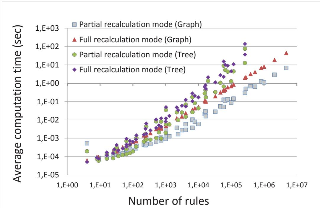
Figure 5: Average computation time in seconds for different rule base sizes in all four modes (log-scale for both axes).
