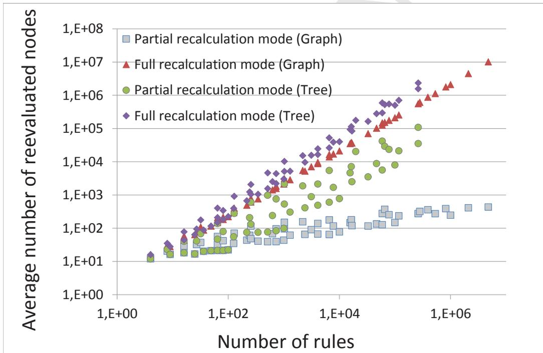
Figure 4: Average number of nodes to be evaluated for different rule base sizes in the all four modes (log-scale for both axes).
