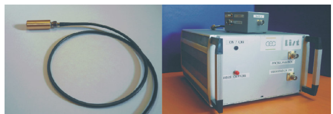
Fig 3. View of the fiber-coupled scintillator (BGO) for the detection of ambient scattered radiation (left) and associated discriminating unit and logic gate (on top) developed by the CEA LIST (right).
