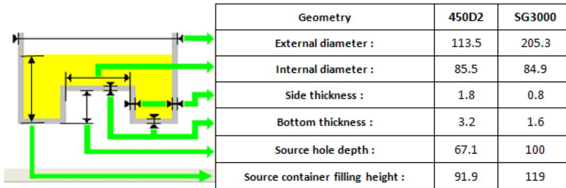
**Figure 1.** Dimensions (in mm) for the Marinelli geometries.
