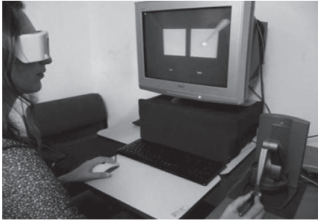
Figure 1. Experimental setup: The right hand holds the PHANTOM's stylus and the left hand is placed on the mouse. Two targets are presented on the computer screen and are seen directly through 3-D glasses. Neither the right nor the left hand is in the participant's visual field while performing the task.
